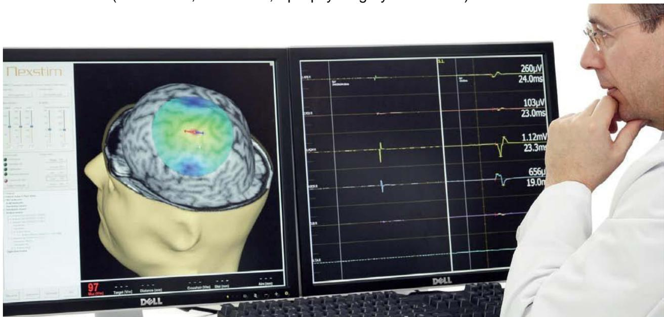
Figure 2: NBS System user interface and stimulation planning screen (left). Location of the E-field maximum is visualized in a 3D rendering of the brain. The 6-channel EMG motor response screen (right) displays online EMG in the right window and triggered EMG responses in the left window.
